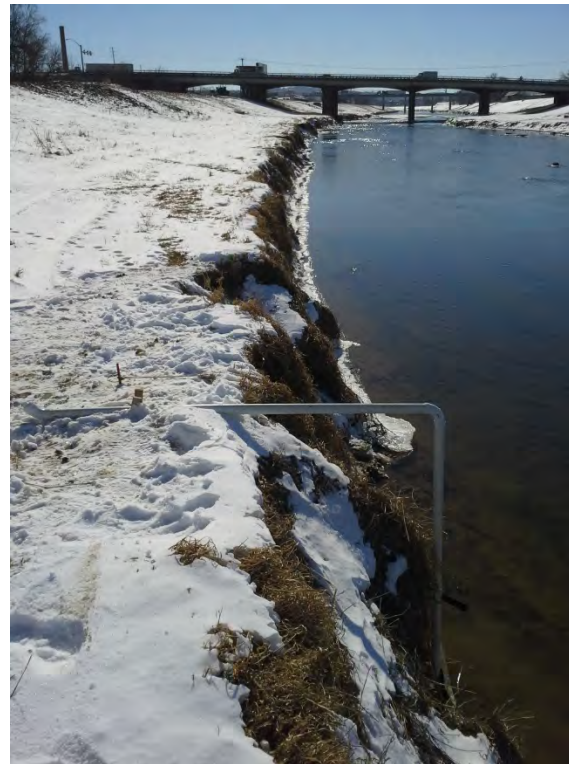
Sampling piping constructed to facilitate SW-17 submerged spring sampling.
