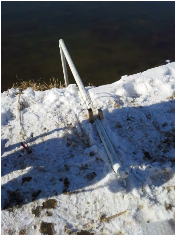
Sampling piping constructed to facilitate SW-17 submerged spring sampling.
